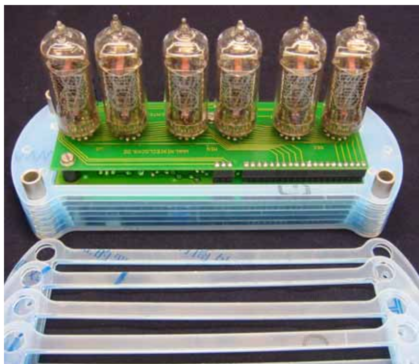
Figure 7 – threading the plates to the aluminium tubes
