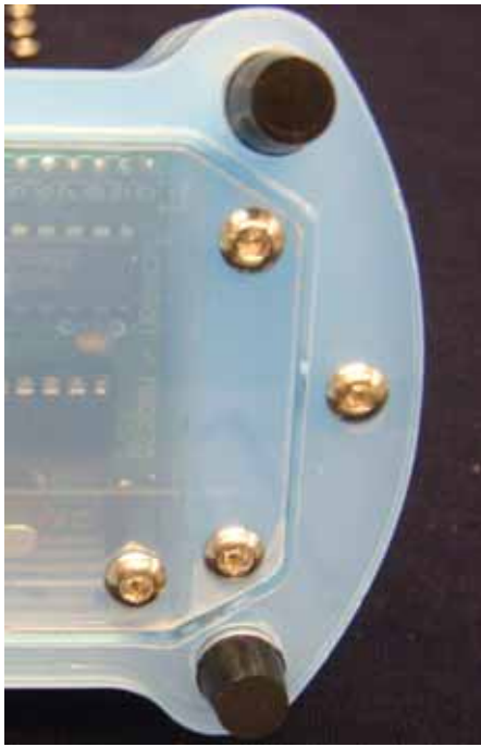
Figure 11 - case bottom screws fit in 3 mm thread
