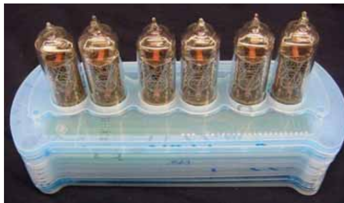
Figure 10 - the tube ring layer- take away the protective foil!
