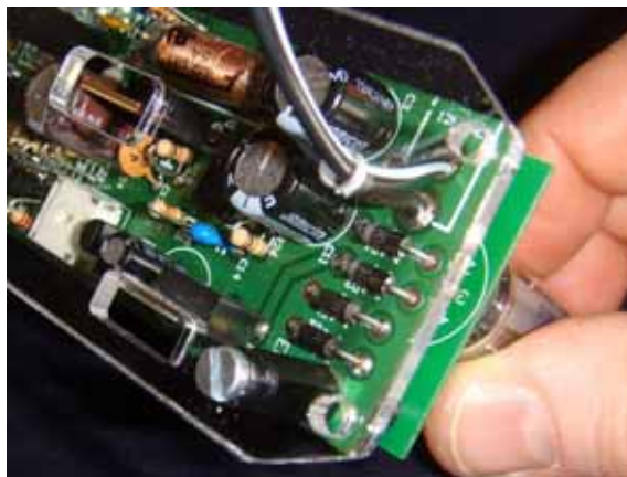
Figure 1 - drilling the hole and solder the cable
