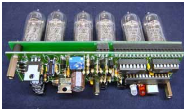
Figure 3 – clock and tube board mounted
