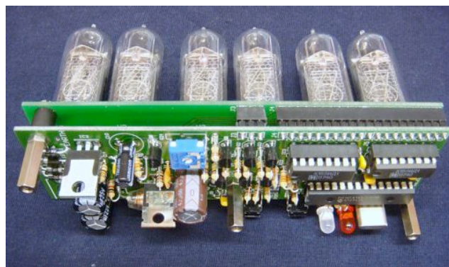
Figure 3 – clock and tube board mounted
