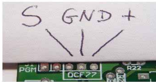
The clock pcb with the important connectors
